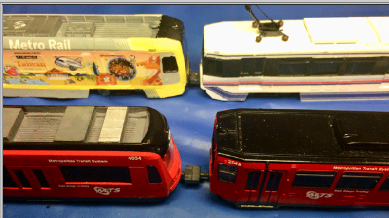
The same four cars, all powered, shown coupled. If mounted correctly and somewhat centered, the couplers will actually find each other and line up correctly for coupling.
