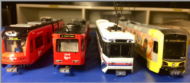
Test versions of the WCTS coupler mounted on HO scale models of a San Diego S70, a San Diego SD100, an Los Angeles P865 and a Los Angeles P3010. The SD100 is a brass model, while the other three are 3D printed.
